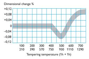
Note: The dimensional changes in hardening and tempering should be added.
