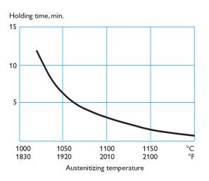
*Note:* Holding time = time at austenitizing temperature after the tool is fully heated through.
